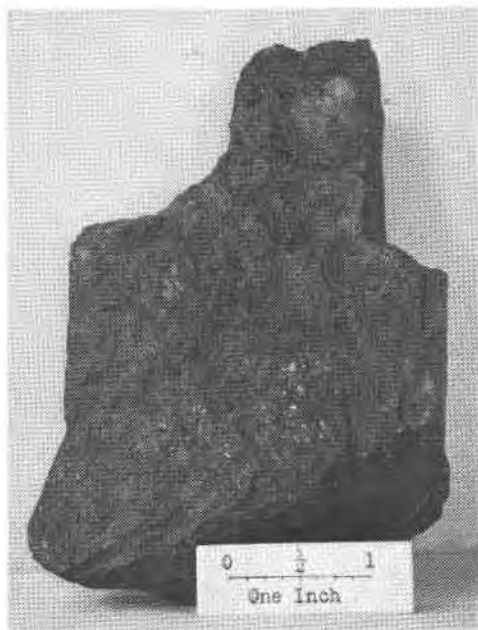
FIG. 3. Photograph of largest monazite fragment found in Yard pegmatite. The shiny spangles are specular hematite.
