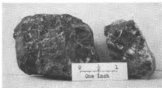
FIG. 4. Euxenite from Yard pegmatite showing fractures filled with typical greenish alteration product.
