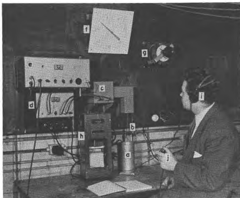
FIG. 2. Photograph of the apparatus in use. (a) Small electric muffle furnace, (b) glass tube carrying the charge, (c) microphone in sound insulating box, (d) audio amplifier, (e) electronic relay, integrating circuit, and power amplifier (f) temperature indicator, (g) variable transformer for controlling the furnace, (h) recording milliammeter, (i) monitoring ear-phones, (j) push switch for producing temperature fiducials on the curve.
