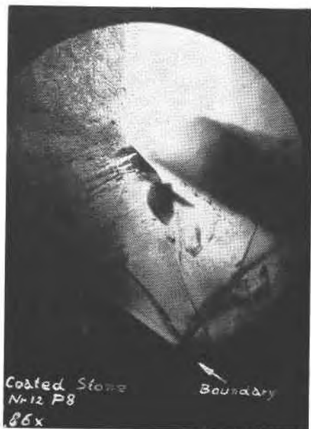
FIG. 1. Boundary between the coating and the clear part of a coated stone. Original magnification on the photograph reduced \frac{1}{2} on reproduction.
