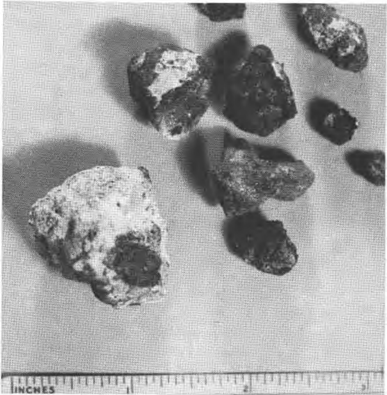
FIG. 3. Collection of nickel-iron inclusions.
