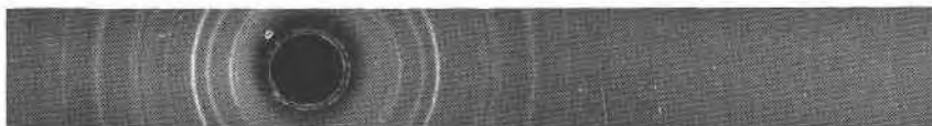
FIG. 1.—X-ray powder photograph, Cu/Ni radiation, 1^\circ\theta=1 mm. on film, actual size print.
