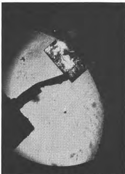
Fig. 4. Photomicrograph of sodium niobate at 560^{\circ} C. Length of crystal: 1.05 mm.
