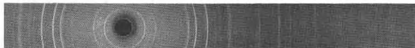
FIG. 2. Kornerupine (yellow variety) X -ray powder pattern, Fe/Mn radiation, Contact print of film from 114.6 mm. diam. camera reduced to \frac{1}{3} size ( 1^\circ\theta=1 mm. on print).
