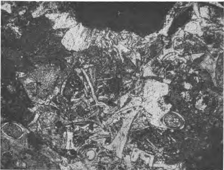
FIG. 1. Laumontitized tuff, no. 8795, North Range, Taringatura Survey District, Southland, New Zealand. A single crystal of laumontite (illuminated) extends right across the field of view, and incorporates many originally glassy ash fragments. These are delineated by dark chloritic films. The shaded region at the lower left and dark regions at the upper left and lower right of the field, represent similar laumontite crystals in near-extinction. Two fragments of twinned plagioclase are also visible. Crossed nicols. \times 60 .
