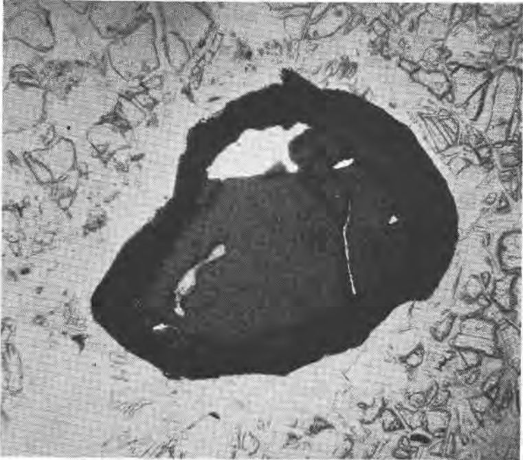
FIG. 4. Chromite grain surrounded by chlorite and partially altered to black opaque material. \times 60
