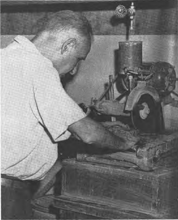
FIG. 2. Use of diamond saw.
