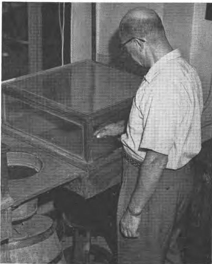
FIG. 1. Grinding unit with horizontal steel lap.
