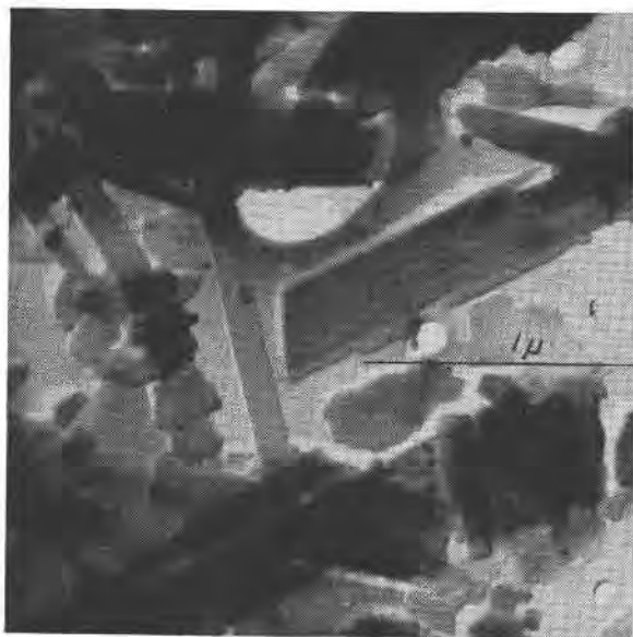
FIG. 4. Electron micrograph of sample OS-8 showing the step-like surface found on many large laths. Mag. 43,200.
