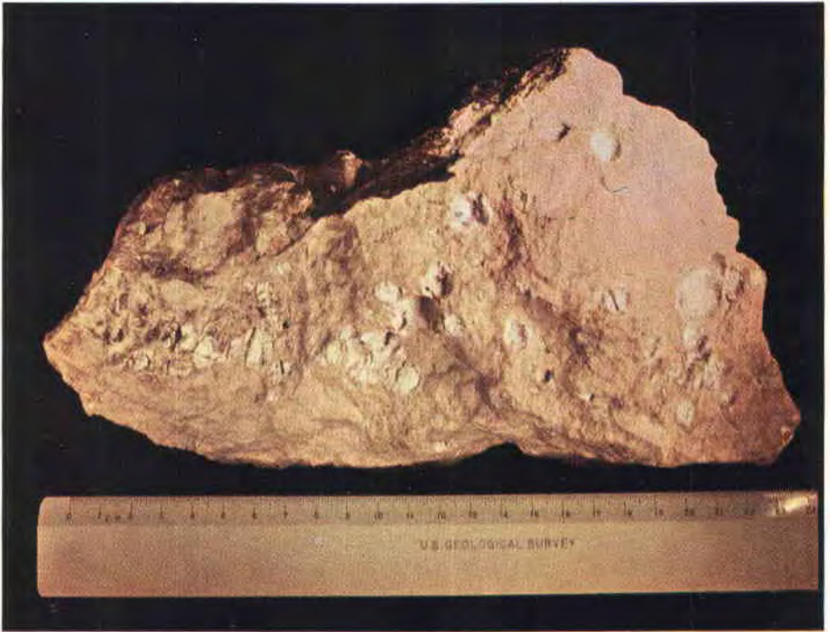
FIG. 5. Replaced tuff N.M.-186. Huntite filling vugs in buff matrix. The matrix is magnesite with some deweylite.
