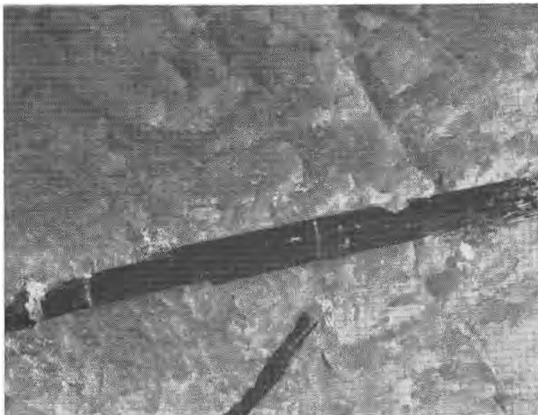
FIG. 17. "Healed-fracture" structure in black tourmaline, Southern Pacific silica quarry, Riverside County, California. The fractures are filled with quartz, which occurs in part as apophyses from the large crystals of quartz that flank the prisms of schorl. The large prism is about 3 inches thick.
