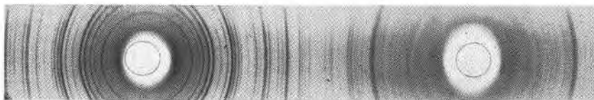
FIG. 1. X-ray powder diffraction pattern of sahamalite taken with a 114.59 mm. diameter camera using Cr K\alpha radiation.
