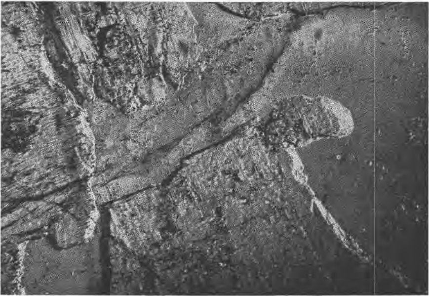
FIG. 9. Highly inclined plane polarized light; mag. 66X. Only quartz, microcline and sericite show in this field of view. This photomicrograph clearly illustrates the great relief differences that can be produced by minerals with relatively small differences in indices of refraction by the use of this technique. A great amount of detail is apparent in both the microcline and quartz. Even the grid twinning of the microcline can be seen under this plane-polarized light. This technique makes it very easy for the petrographer to distinguish by inspection between quartz and orthoclase—a feat not always easy under ordinary circumstances—and hence greatly increase the precision and speed of making grain counts without having to resort to tedious and frequently unsatisfactory staining techniques.
