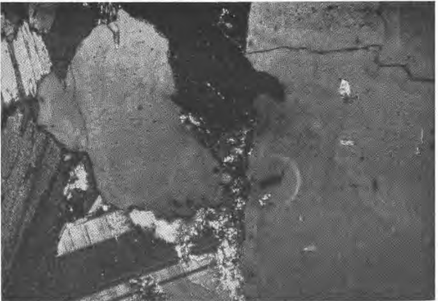
FIG. 8. Same as 7 except taken under crossed nicols. The channels transect both quartz and oligoclase. Small relief ridges remain on parts of the plagioclase.
