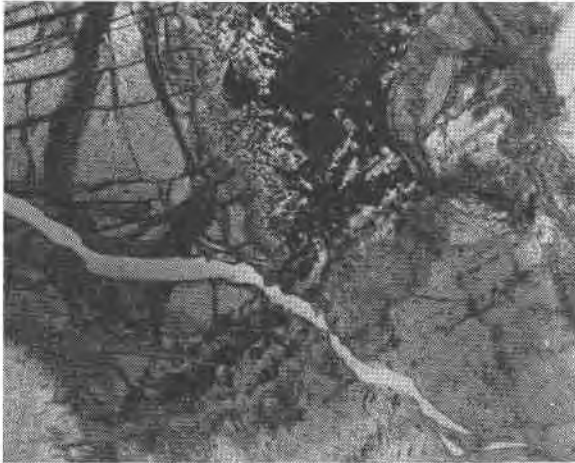
FIG. 2. C-142, plane light \times 58 . Olivine is surrounded by a corona built against anhedral of plagioclase An_{76} . The reaction products are composed of two shells. Close to the olivine is a shell of hypersthene. This shell passes outward to a diopside-spinel symplektite. Note a part of the olivine is selectively replaced by iron ore.
