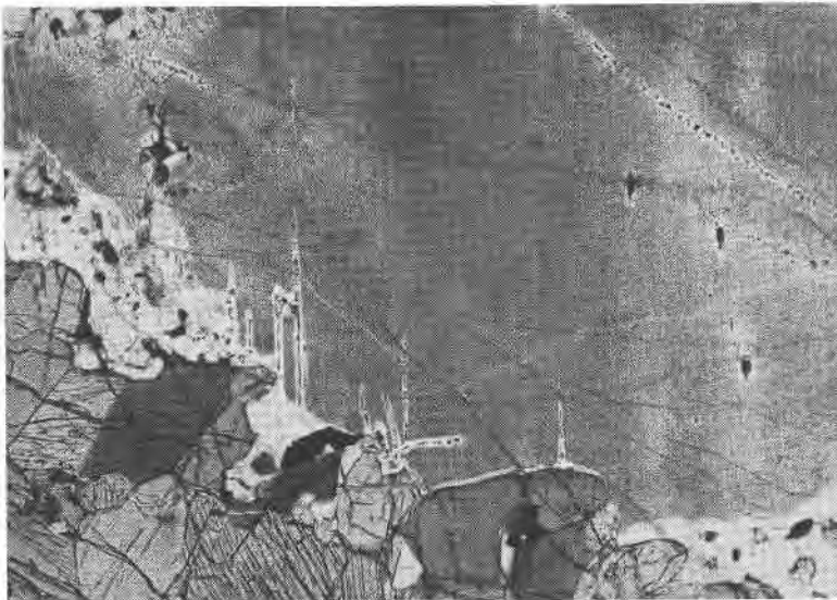
FIG. 2. Magnetite-ilmenite ore, Sanford Lake, Adirondack Mountains, New York. Clouded plagioclase crystal with trails. Note cleared incursions with larger microlites extending inward from unclouded periphery. \times 25 .
