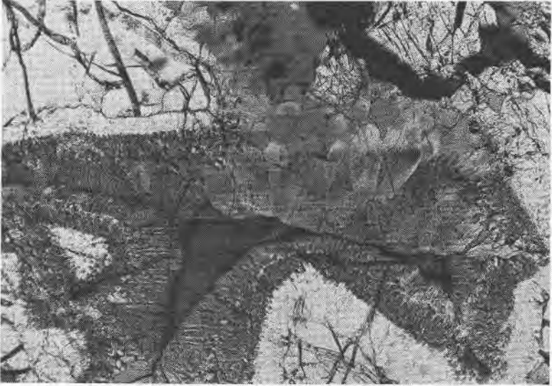
FIG. 5. Coronite, eastern Quebec. Corroded plagioclase crystal with spinel and opaque ore particles which extend into the surrounding hornblende corona. \times 30 .
