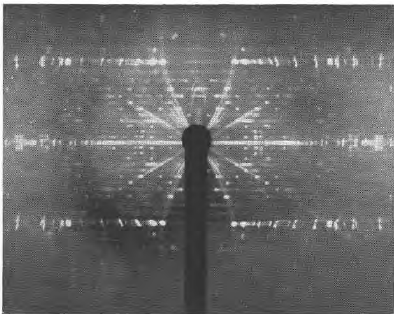
FIG. 3. Rotation diagram of ekmanite taken with rotation around the b axis. Fe K_{\alpha} radiation. Most of the weak, diffuse reflections were lost when a reversed (negative) print was made from the original rotation photograph; a positive print of the x -ray film, that is shown above, is in good agreement with the original pattern.
