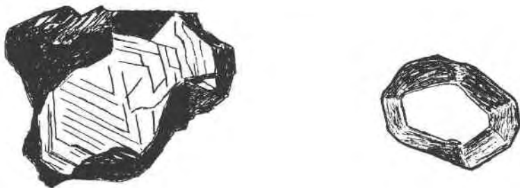
FIG. 2. Left —Yellowish-green crystal of pyrophanite oriented with the dominant face (0001) parallel to the plane of the preparation. Such crystals give centered interference figures and exhibit (11 \bar{2} 0) and (02 \bar{2} 1) cleavages. Locality: Ajiro mine. \times 570 . Right —Orange-red crystal of pyrophanite. The euhedral tabular form is typical of many crystals from all six mines described. Interference figure about 5° off center. Locality: Kusugi mine. \times 570 .
