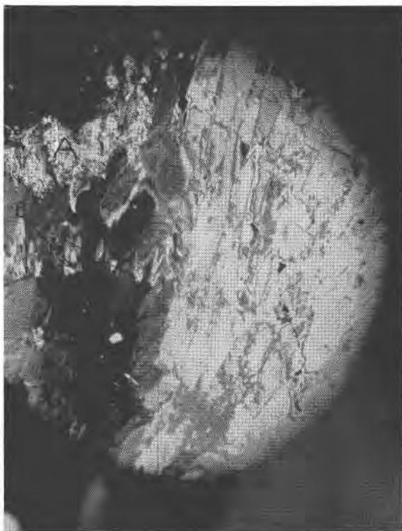
FIG. 1. Portion of spherulite showing radial arrangement of wavellite crystals. Part of concentric structure marked by cryptocrystalline sheaves of wavellite at B . Partly replaced phosphatic cement in upper left at A . Crossed nicols, \times 70 .
