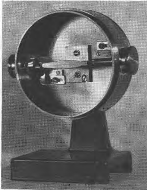
FIG. 2. Front view of camera, showing central slit system, ring shields for limiting angle of reflection (one retracted), rotating sample holder (left) and shield for end of inlet slit (right).
