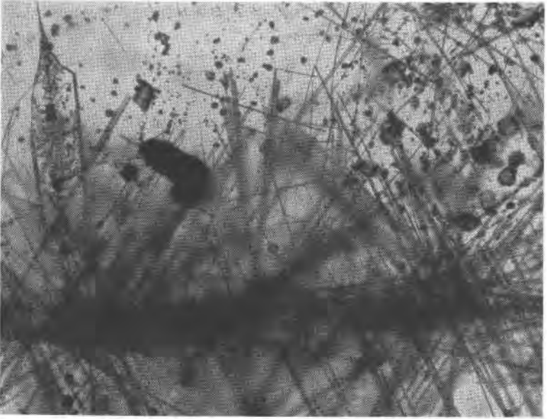
FIG. 4. Needles of diaspore radiating into the muscovite from a scratch in the surface. Smaller equant crystals are boehmite. In plane-polarized light, \times 107 .
