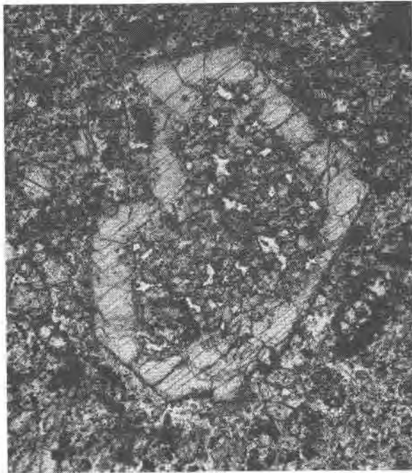
PLATE 5. Augite phenocryst with vesicular core. The vesicles are filled with sanidine. Picture area is 2 mm. long. Ordinary light.
