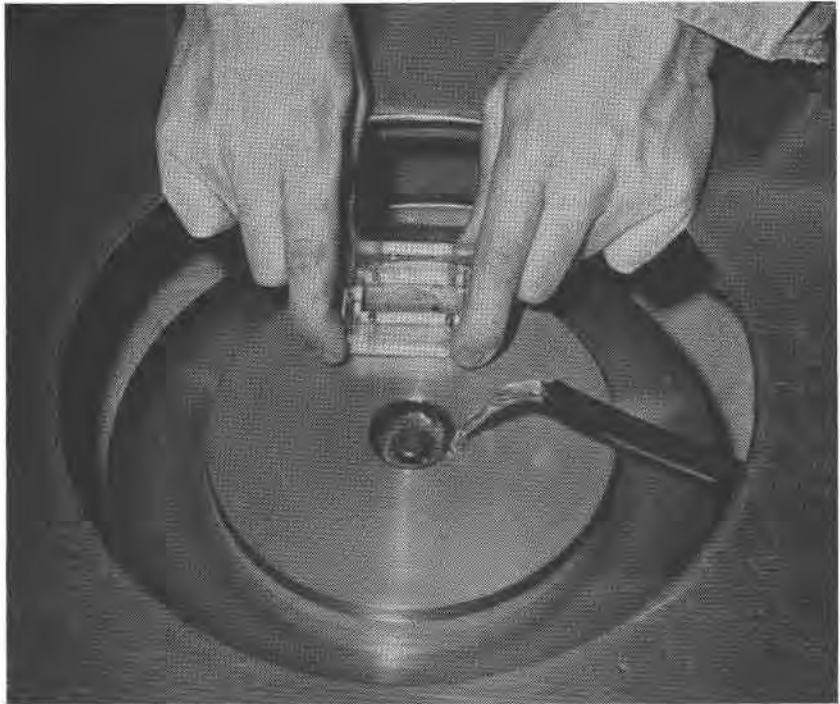
FIG. 1. Close-up of bonded diamond wheel in use. Note the special slide holder, and the freely flowing stream of water.
