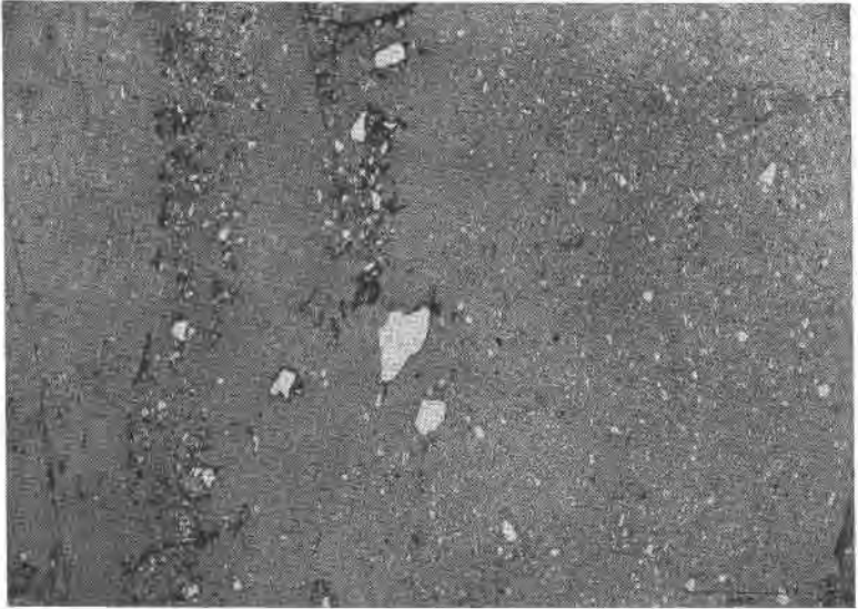
FIG. 2. Thin section of nodule, such as shown in Fig. 1. The white areas are quartz, the dark spots are light brown organic (phosphatic) material. The gray matrix is gorceixite.
