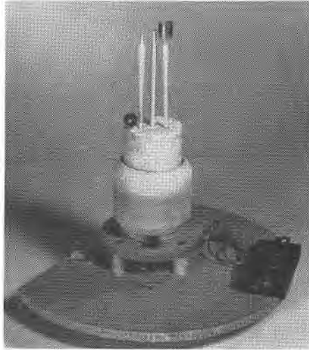
FIG. 1. DTA sample holder. External thermocouple assembly.
