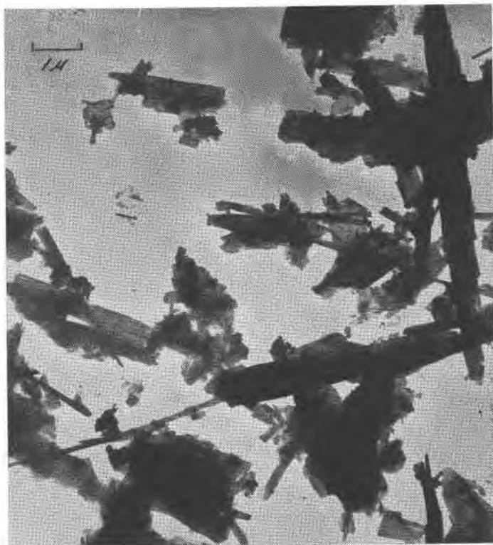
FIG. 1. Electron photomicrograph showing lath-like structure of chromian antigorite from the Wood's mine, Lancaster County, Pennsylvania.
