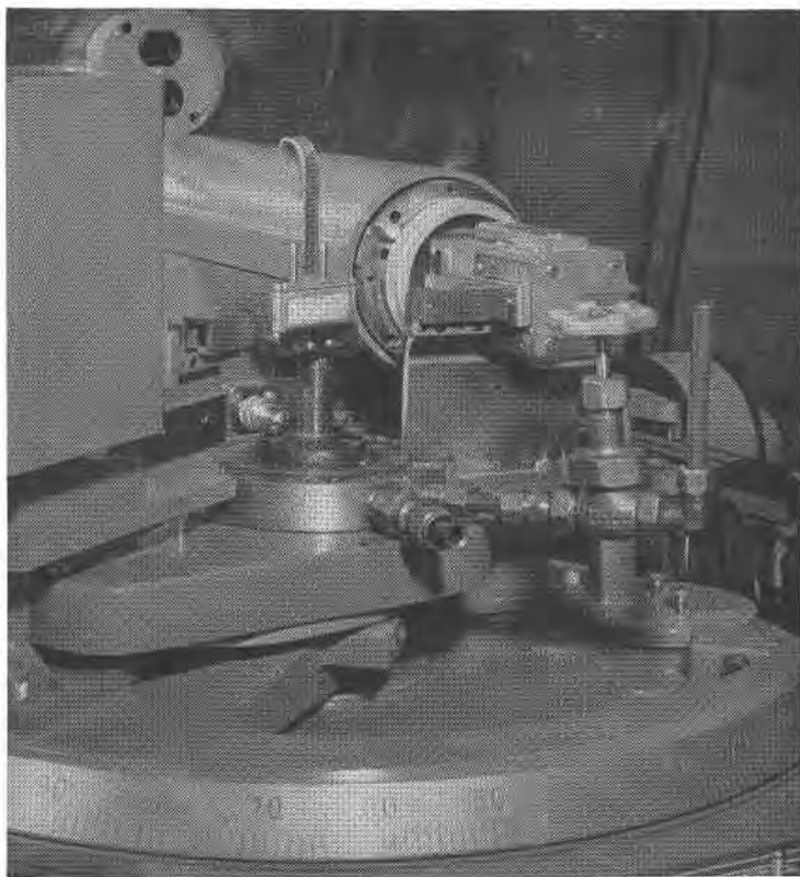
FIG. 2. Sample stand and sample holder for autoclave unit.
