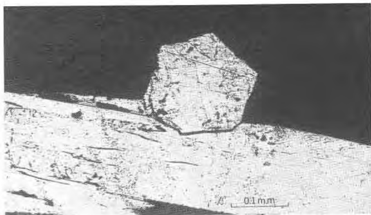
FIG. 10. Polished section showing cross and longitudinal sections of twinned millerite crystals. The twinning is brought out by natural tarnish in the laboratory.
