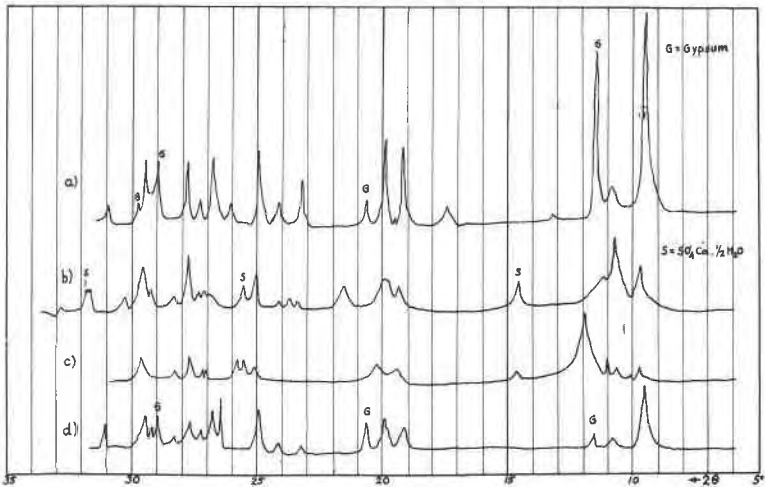
FIG. 4. X-ray diffraction goniometer traces of impure ranquillite.
