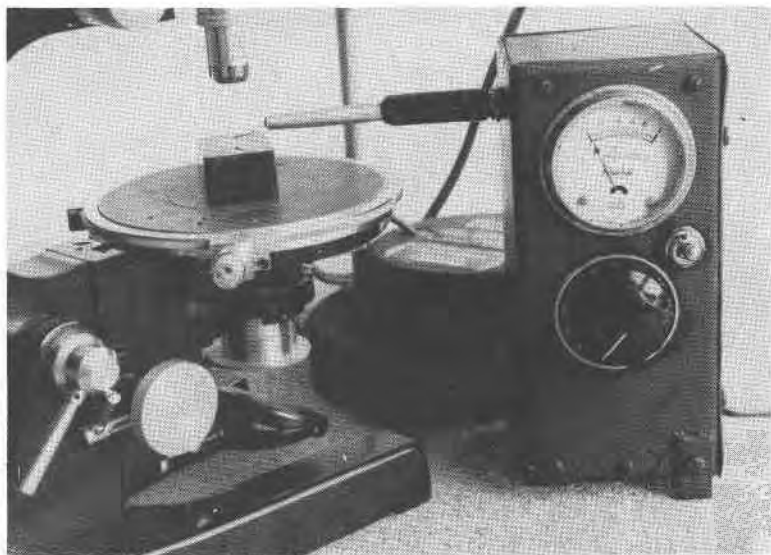
FIG. 1. The micro-coil in position for heat-etching of a polished section.
