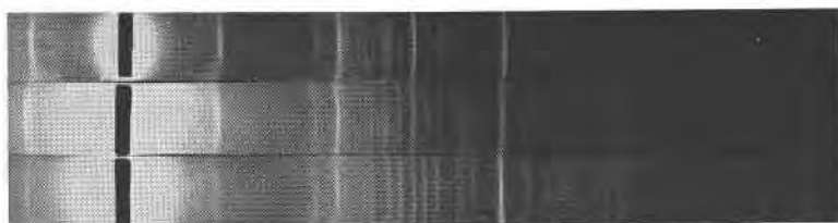
FIG. 1. X-ray powder photographs. (Above) 2:1 mixture of 1M muscovite and 2M_1 muscovite, ( d ). (Middle) Hydromuscovite from Mt. Lyell, Tasmania, ( a ). 2M_2 lepidolite ( e ).
