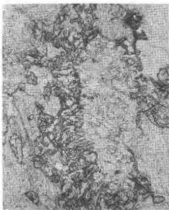
FIG. 11. Apatite grain with dactylic overgrowth of monazite in Sr-Ba calcite (II). Sheep Creek vein. 42X.
