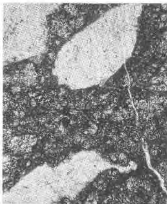
FIG. 5. Corroded remnants of Sr-Ba calcite (II) in fine-grained ancylite quartz aggregate. Late veinlet of calcite (III) cuts both. Sheep Creek vein. 70X.
