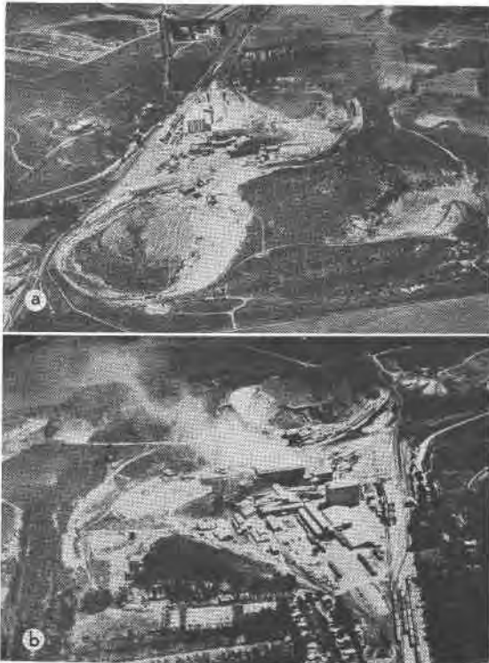
FIG. 2. Crestmore in 1928. (a) View from East, showing old Commercial quarry face, and old lime kiln structures. (b) View from West, showing the high Lone Star quarry and greatly deepened Wet Weather quarry.
