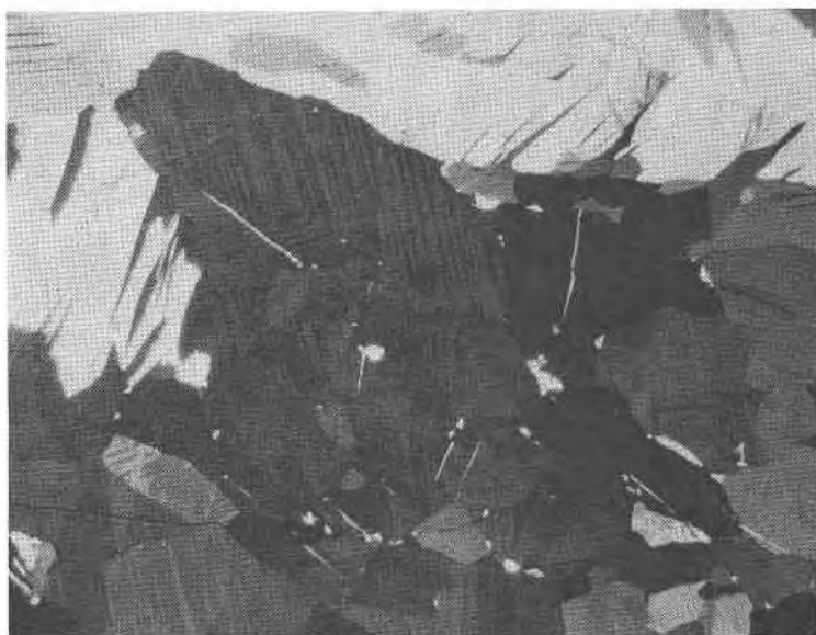
FIG. 5. Rickardite (medium to dark gray), showing complex twinning. In the large crystal in the upper half of the field a thin blade of vulcanite (white) is oriented at about 45^\circ to the twinning, but other blades show variation in orientation. White to light gray grains are vulcanite. Crossed nicols, \times 140 .
