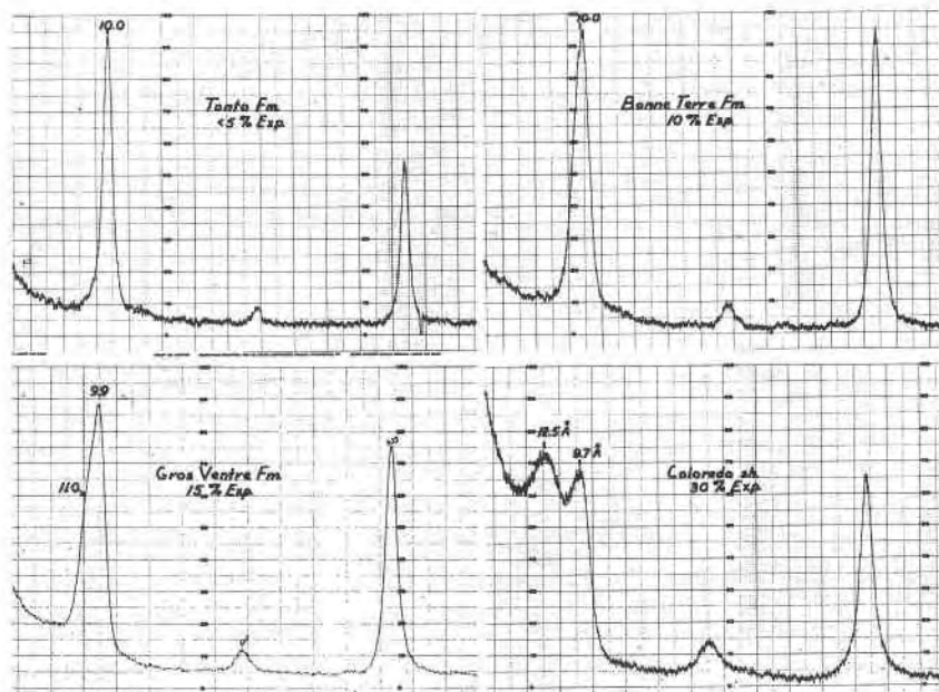
FIG. 1. Examples of monomineralic glauconite pellets composed of mixed-layer illite/montmorillonite. The samples are glycol solvated. (upper left) Tonto Fm., Cambrian, 5% expandable layers, 6.7% K; (upper right) Bonne Terre Fm., Cambrian, 10% expandable layers, 6.9% K; (lower left) Gros Ventre Fm., Cambrian, 15% expandable layers; (lower right) Colorado shale, Cretaceous, 25% expandable layers, 4.2% K.
