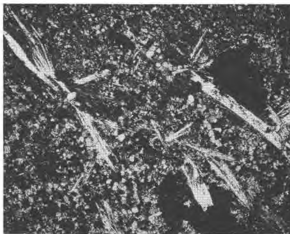
FIG. 1. Metamorphosed manganese carbonate rock from Nsuta, Ghana, showing acicular-prismatic manganoo cummingtonite in a matrix of granular calcian, magnesian rhodochrosite, quartz, and spessartite. Crossed nicols \times 30 .
