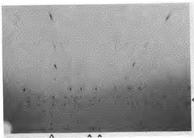
FIG. 4. One quadrant of c -axis rotation pattern of davidite, Arizona Co-Fe, 16 hours. Arrows indicate features discussed in text.
