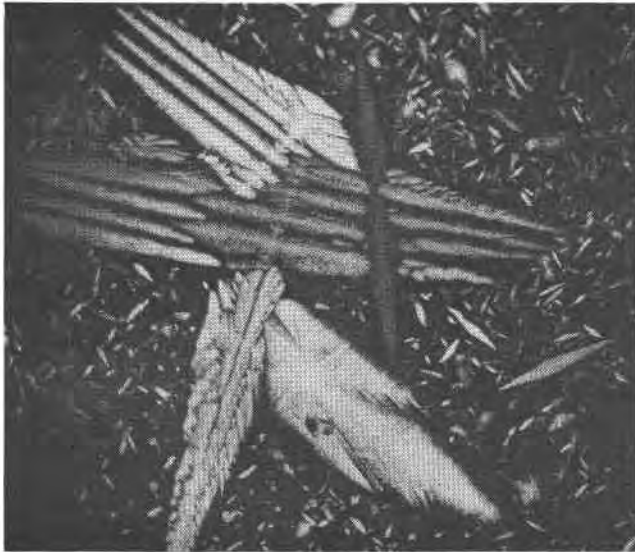
FIG. 1. Slag with silica/lime ratio of 0.67. Cooled in six hours to give a glassy matrix with skeletal phenocrysts of cuspidine. Crossed nicols. \times 35 .
