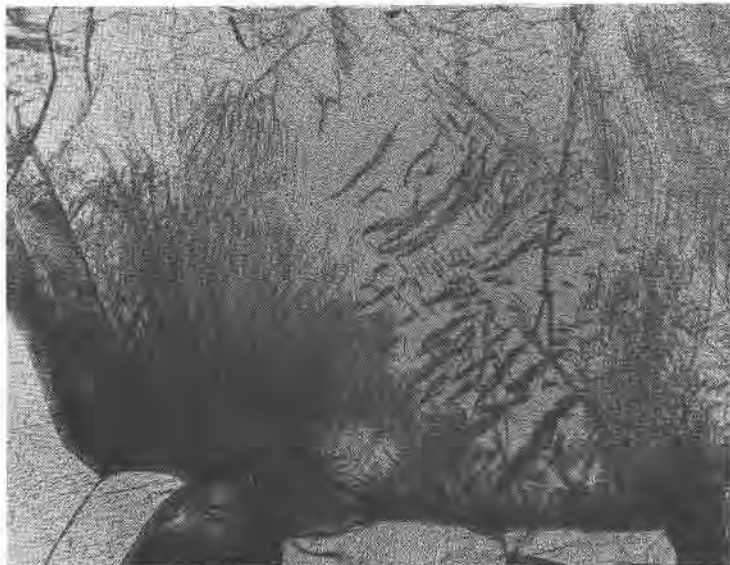
FIG. 6. Photomicrograph of an olivine exsolving iron ores. Specimen X11A, Gough Island. Note the difference in appearance between this and the "iddingsite" shown in Fig. 5. Ordinary light, magnification \times 65 .
