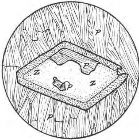
FIG. 2. Zoned zoisite crystal (z) selectively replaced by phlogopite (p). From scapolite rock at margins of aplite dike, Metronite quarry. 50x.
