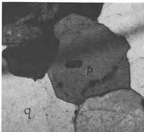
FIG. 6. Photomicrograph showing facets of the grain p interfering the overgrowth of the grain q; crossed nicols, \times 100 .
