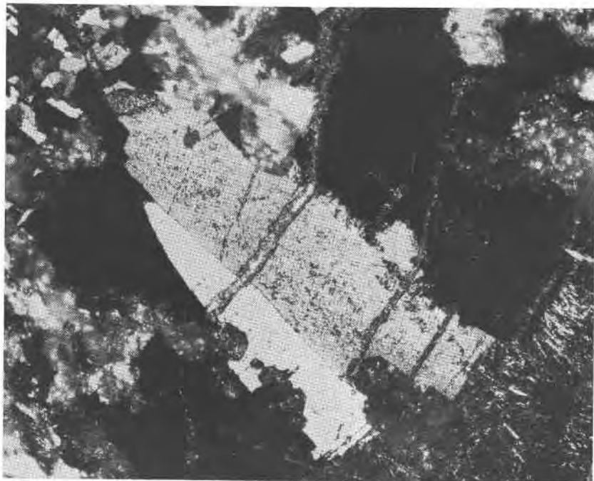
FIG. 1. Photomicrograph. Large cryptomelane grains that occur interlayered with jasper in the Black Jack deposit. The cloudy and unevenly highlighted gray and white material is quartz. Partial outlines of quartz crystals may be seen in places along the edges of the cryptomelane grains. 370X. Crossed nicols.
