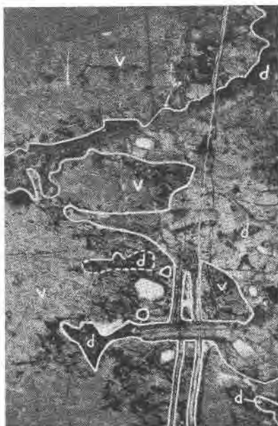
FIG. 5. Photomicrograph of irregular contact between vitrophyre (v) and "dike" of devitrified rock (d). Textures on both sides of the contact are essentially identical except where the original texture has been destroyed by growth of incomplete spherulites, as along the upper right-hand segment of the contact. Plane polarized light, \times 33 .
