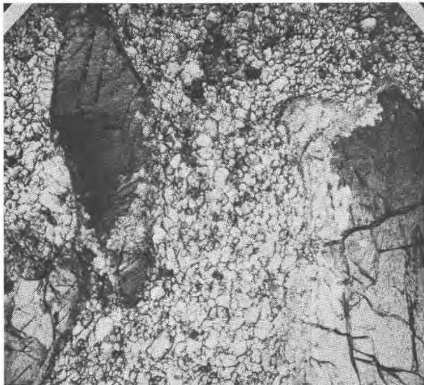
FIG. 3. Ultrabasic nodule E3 showing mortar texture. Note the irregular extinction of the well-cleaved olivine grains. Crossed polars ( \times 40 ).
