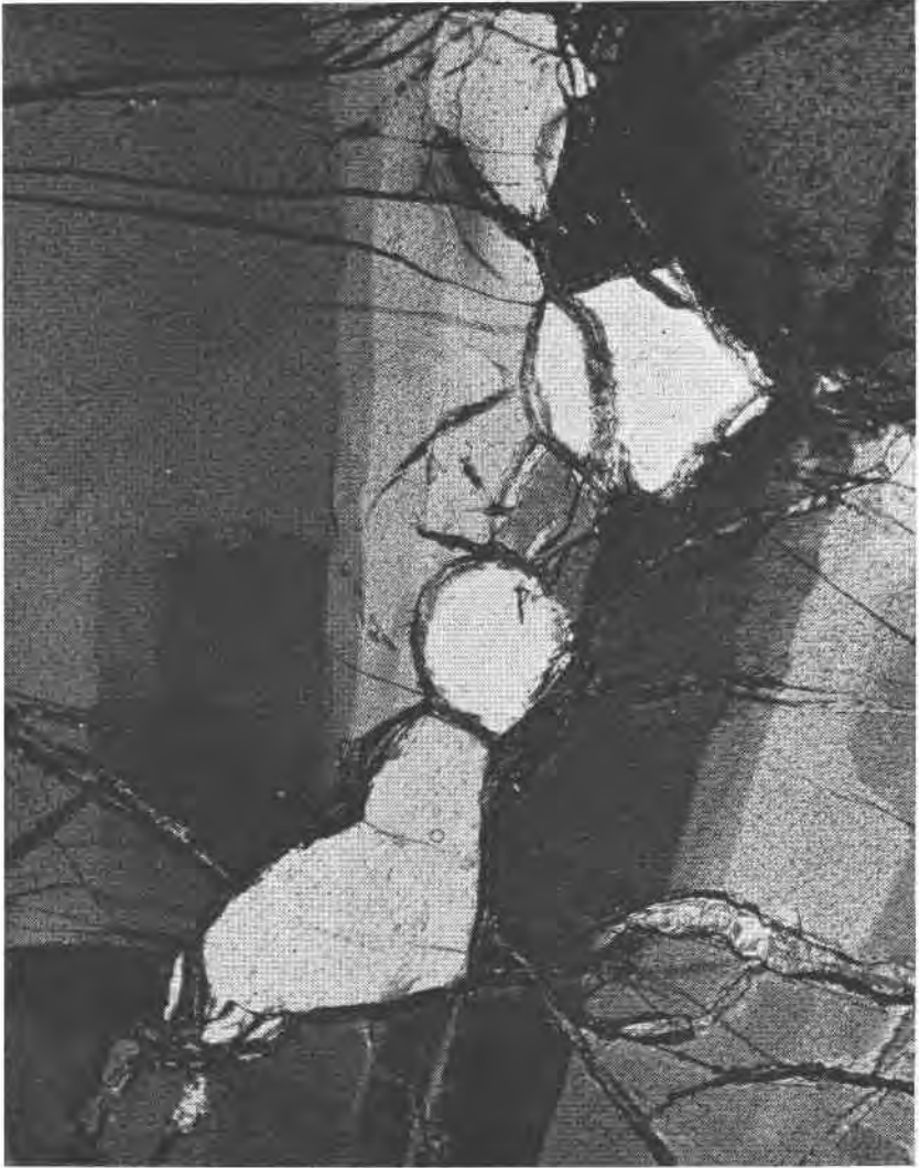
FIG. 2. Polygonal grains of olivine adjacent to a large strained olivine grain. Crossed polars (K29). Height of area 2.6 mm.
