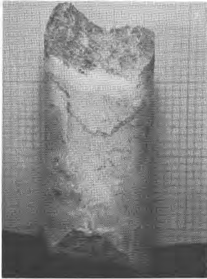
FIG. 1. Specimen of drill-core with small crystals of cymrite (black flakes) scattered through a dolomite breccia. Pyrite-filled stylolite and a veinlet of calcite are also present. Small squares equal 0.1 inch.
