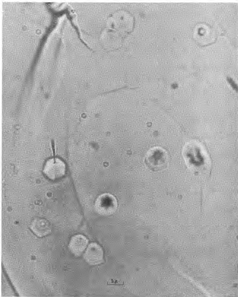
FIG. 1. Etch pits on the basal plane surface of an apatite crystal etched in concentrated nitric acid for 25 seconds at room temperature.
