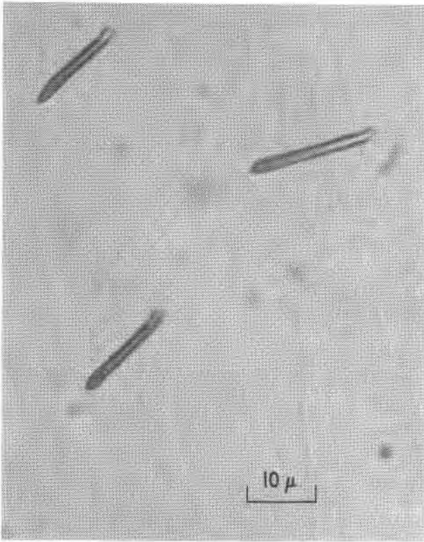
FIG. 3. Fission fragment tracks in mica. The same three pits as Fig. 2, but after an initial etch of only 20 minutes in concentrated hydrofluoric acid at room temperature.
