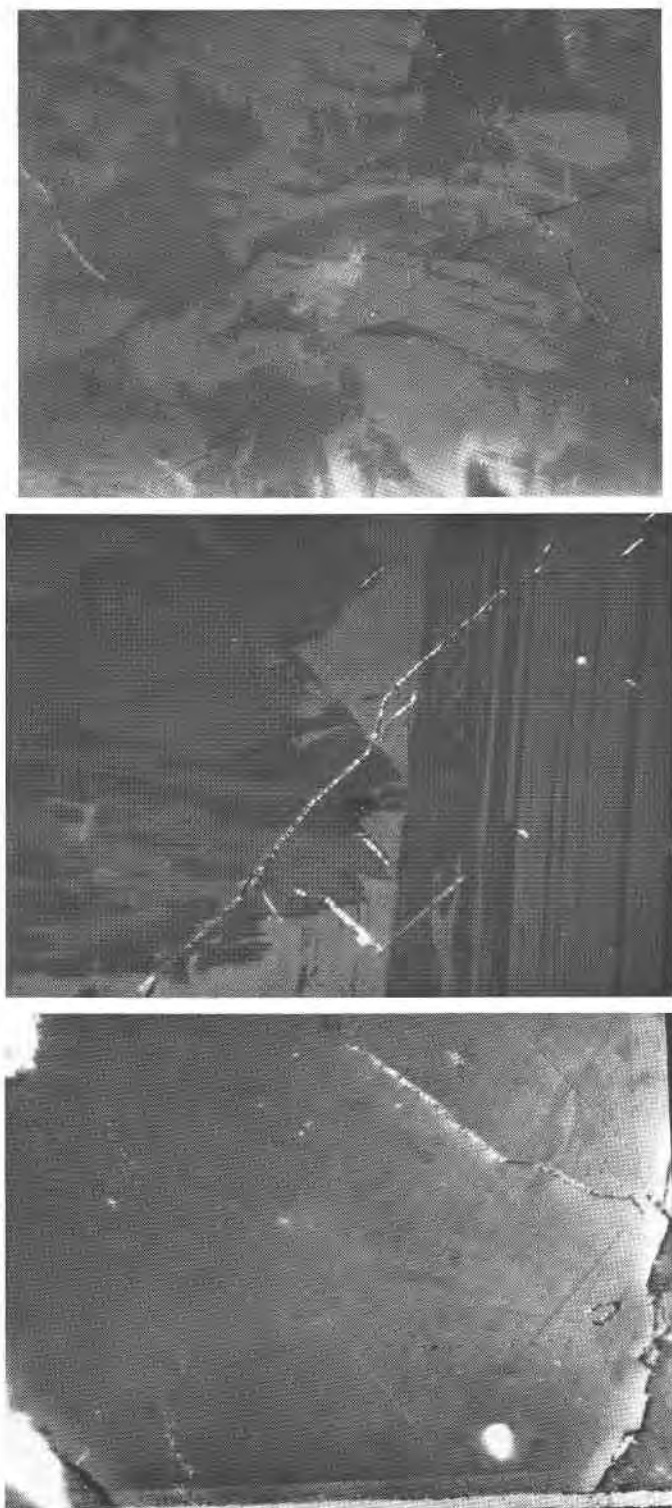
FIG. 2. Polished section photographs of cobaltite (150X). Figs. 2a, b—natural material. Fig. 2c—material quenched from 850°C.
