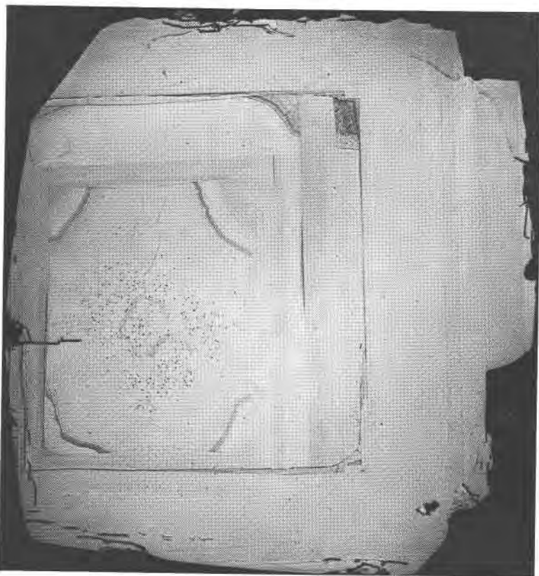
FIG. 5. Diamond no. 534A (Kimberley, type 1). The section is approximately through the center of the diamond, and at the edges it intersects curved and fractured dodecahedral faces. Magnification 28\times .
