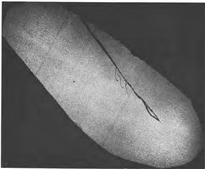
FIG. 18. Diamond no. 772A (Premier Mine, type 2A). This diamond had an irregular shape, flattened at one end and elongated to a point at the other. There were many curved and twisted faces. This etched section passes across the flattened portion. Magnification 28X.
